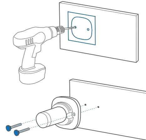
3. Firmly screw the knob of the mounting bracket into the mounting hole.
