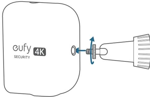
4. Hold and screw the camera to the mounting bracket. Rotate the camera to adjust the view and check it using the live stream, which you can access in the eufy Security app.
