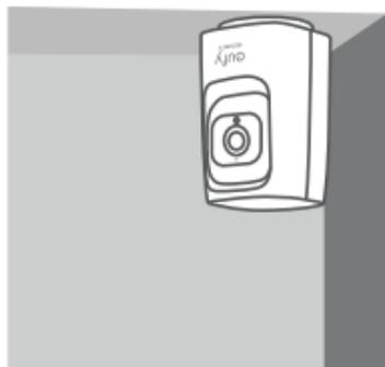
💡 Keep the camera at least 0.7 ft / 20 cm away from walls or anything that may obstruct the view. Do this to avoid infrared reflection which can have a negative impact on the night vision performance.
